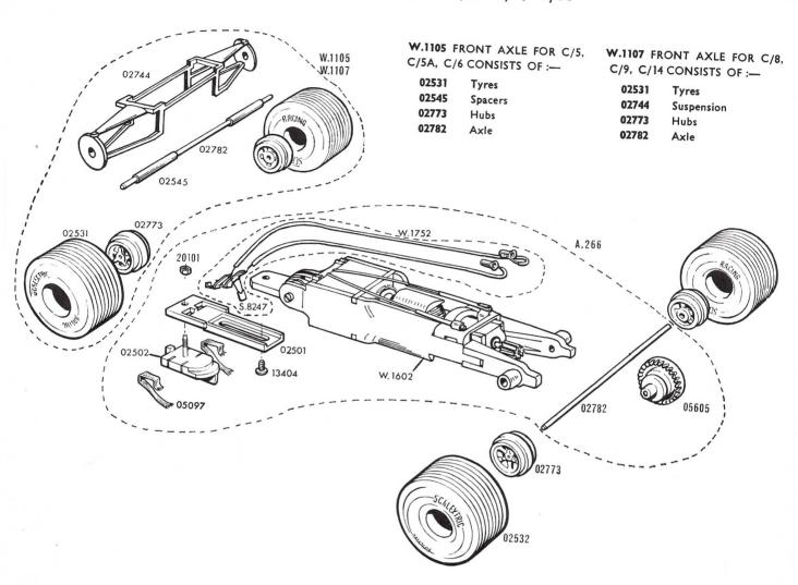
Complete Power Sledge Front Axle Assembly W.1105 W.1107 Front Axle Assembly Motor W.1752 Wiring Harness Capacitor
